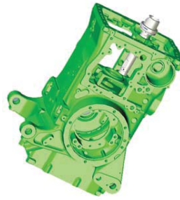
Example of tractor gearbox with deeper cavities needing AV holders
